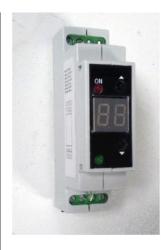
The CRE1 module allows setting a setpoint through its displays and pushbuttons and activating a relay depending on the state of the input signal (higher or lower than setpoint, window between two setpoints ...). The value of the input signal is displayed on the displays. Two relays with combined functions can also be activated. Mounts on DIN rail.
