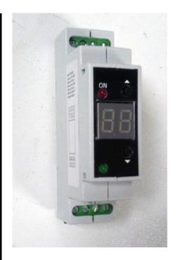
The SC module allows a directional current of up to 10A to be measured inside an electrical panel, in a reduced size by means of a Hall effect sensor with 2KV isolation. The current is visualized on a two-digit display and a setpoint relay (SPST) can be configured to set a setpoint using its pushbuttons as well as relay on and off delays. It has analogue output 0-10V, 4-20mA or in ModBus RTU RS485 communication Mounted in box for DIN rail.
